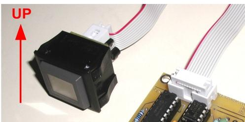
We provide an 18 inch long interconnecting ribbon cable to connect the Display/Button to the Input/Driver board. When connecting these two boards together, please pay attention to the location of pin 1. Orient the banded side of the ribbon cable towards pin 1 on both boards. Pin 1 is marked on both boards. If the cable has no banded side, use the pin 1 designation on the connector for this indicator. ***NO WARRANTY repair if you mistakenly connect the display backward, sorry!***
